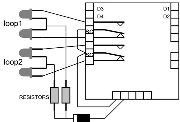
The internal relay contacts are shown as thick lines. "sc" is the common to which one wire of the signals power connects. This is switched to one of the adjacent terminals by the SA5-S to
