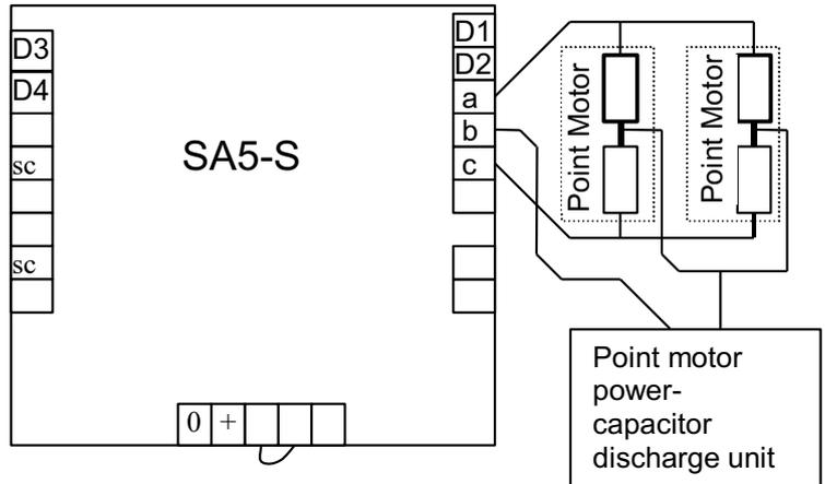
the end of the first passing loop. The train will stop and the red and green lights flash alternatively then the train will accelerate away. On the second lap, D3 will again slow the train but D2 will halt it, as the points would now have set for the second loop. Check the IRDOT-1s are wired correctly by placing your hand over the detectors in the same order. Note that the detectors must operate in the correct sequence. A train must operate D3 before it can be stopped by D1 or D2.
