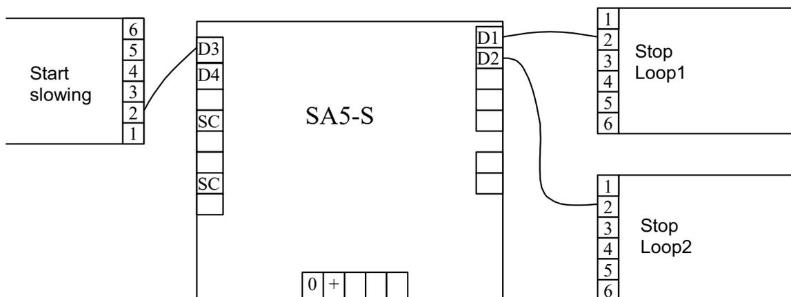
terminal 2 of the loop 1 IRDOT to D1. Wire from terminal 2 of the loop 2 IRDOT to terminal D2.
