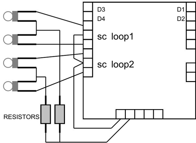
**POWERING FROM 16 VOLTS AC:** The SA5-SB and IRDOTs can be powered from 16 volts AC. This requires the link wire to be replaced by a diode. The band on the diode must be in the direction shown.. If AC is used the output at the track will be half wave rectified DC. If a 12-volt DC supply is used the output at the track will be pure DC. The capacitor can be used. This will smooth the DC. The side of the capacitor with the minus signs and arrows must connect to the terminal shown.
