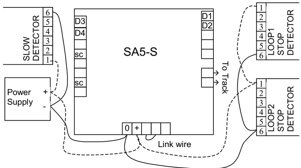
The first diagram shows the track wiring for electro frog points. Power is fed to the track so that trains are isolated by the points setting.
